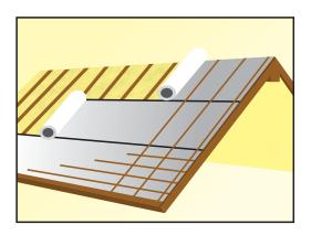
This insulated roof underlay product is a laminate made from a low emissivity reflective membrane and white polyester insulation. The reflective side should be installed facing to the outside of the construction. The first layer should be unrolled parallel to the bottom of the roof. The lap joint with the integral adhesive tape strip always faces down.
