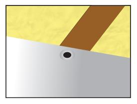
Temporary attachment is then made about 30mm from the upper edge of the lap joint by means of suitable BS 5543 fixings. Battens or counter battens are fixed permanently later on during the installation process.
